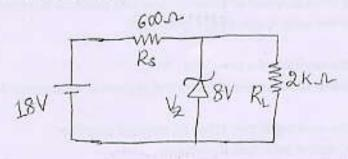
12. For the given circuit, locate Q point on the DC load line.
