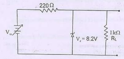
12. Determine the coordinates of Q point for the circuit shown.
